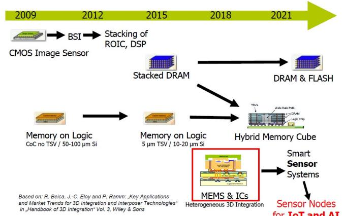
**Figure 3:** Roadmap for 3D IC application development
