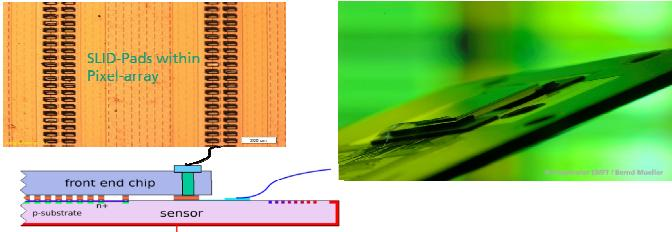
**Figure 5:** Heterogeneous integration of detector and readout circuit (Fraunhofer EMFT in co-operation with Max-Planck)
