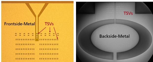
**Figure 6:** Micrograph (left side) and SEM-picture (right side) of 3D-TSV integrated antenna structure for 60 GHz.
