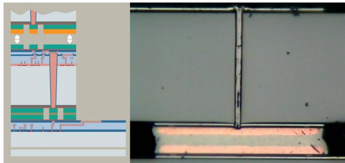
**Figure 2:** Application of wafer bonding for 3D IC integration: TSV-SLID technology based on metal bonding by Solid-Liquid-Interdiffusion (SLID) [9]
