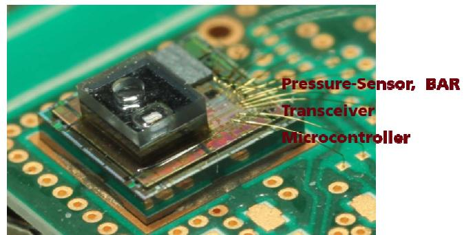
**Figure 4:** 3D heterogeneous system for tire pressure monitoring (Infineon, Fraunhofer, SINTEF)
