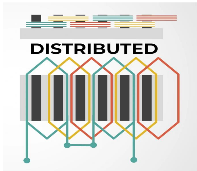
Figure 19 Schematic and winding diagram of distributed winding [16]
