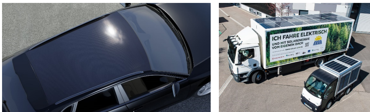
Figure 1. Solar roof design for cars built at Fraunhofer ISE (left), and concept truck equipped with VIPV modules on the roof (right).
