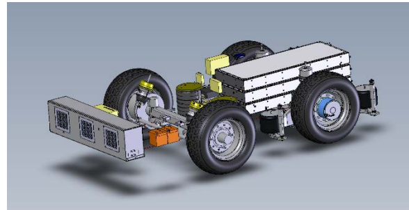
Fig. 9: CAD model of the SPD reduced to the electric powertrain components (driven axle, battery, inverters), steered axle, cooling system and ECUs
