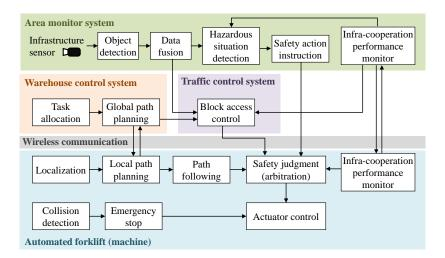
Fig. 2. Infrastructure-Cooperative Autonomous Control Architecture
