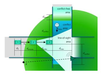
Fig. 1. An automated forklift approaching a blind corner.
