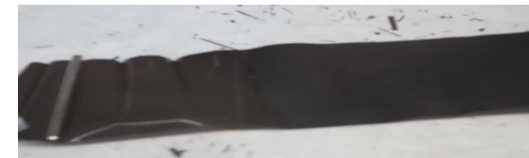
LiFePO<sub>4</sub> /C cathode - Center of battery cell
