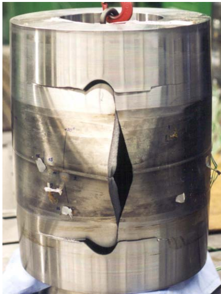
Fig.13: Sub-scale pressure vessel No.2 with surface defect after burst test and comparison of experimental and calculated burst pressures
