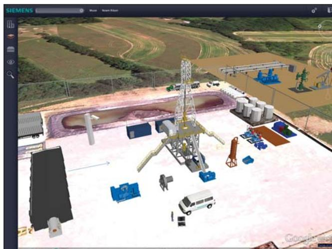
Figure 8: For each piece of equipment, IntoSite is displaying on Google Earth updated information, including 3D representations
