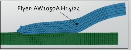
V109: 30kJ, 544kA, 22.2kHz, t<sub>flyer</sub>=2, gap=3, x=-2
