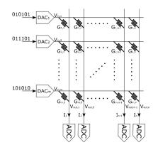
Fig. 1. The basic concept for crossbar implementation of matrix-vector multiplication, which might be used for the dense layer in our design. The DACs convert the digital signals from the convolutional layer to analog voltages, and the multiplication can be performed by applying the ohm's law for every programmable resistor (memristor). The resulted current is the product of the multiplication. If required, the output current can converted back to digital value by using ADCs.
