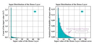
Fig. 5. The inputs of dense layer are collected. (a) shows the original distribution of values, that most values are located at 0. Then, all zeros are removed. (b) input values (without zeros) exhibit an exponentional distribution. The purple line is the resolved exponentional function.
