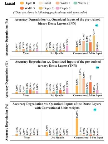
Fig. 6. The proposed quantization is used for inputs of the dense layer with different configurations. (a), (b) and (c) compare the accuracy degradation of the CNNs if those methods are applied to original pre-trained binar (BNN), ternary (TNN) and conventionally 3-bits quantized dense layer of CNNs. It results in that a fully 1-bits (both inputs and weights) dense layer of the CNN can be achieved by using porposed method and only litte accuracy degradation occurs for MNIST Dataset.
