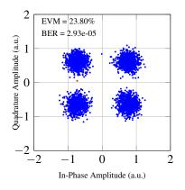
Fig. 3: Constellation plot of received 1.625 GBit/s QPSK signal transmitted over 800 m free-space link. A single bit error (red point) was measured in the transmission of over 34000 bits.
