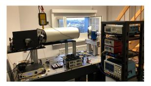
Fig. 1: Schematic and image of the optical hardware used in the transmitter and receiver. HWP = Half-Wave Plate, QWP = Quarter-Wave Plate, OBPF = Optical Bandpass Filter.
