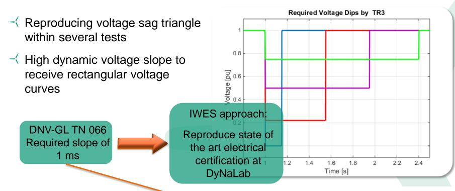
The voltage drop can be achieved with a reactor by short-circuiting of two and three phases at the turbine side of the impedance. The test set up according to IEC 61400-21/4/, section 7.5 can be used (two reactors Z1 and Z2 as a voltage divider). The voltage drop should be accomplished in 1 ms fall time of the signal from  $U_n$  down to User at the beginning of the drop – otherwise as fast as possible – so that a short circuit in the grid is reproduced close to reality.
