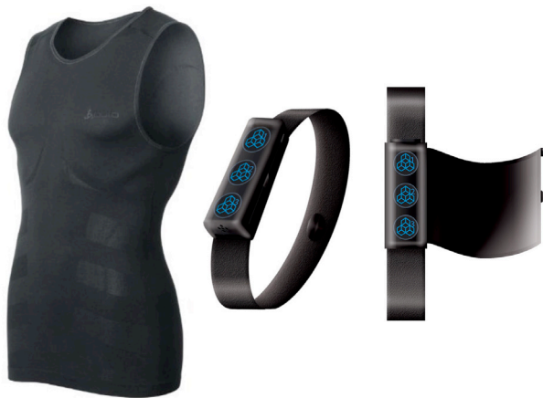
Figure 8. The envisioned system would consist of a shirt and an arm-band. A shirt can be worn under everyday clothes while it would incorporate feedback modalities such as vibration and heat. The wrist-worn device would enable the user to run and adjusted individual relaxation programs, while an expandable OLED display allows for complex input.
