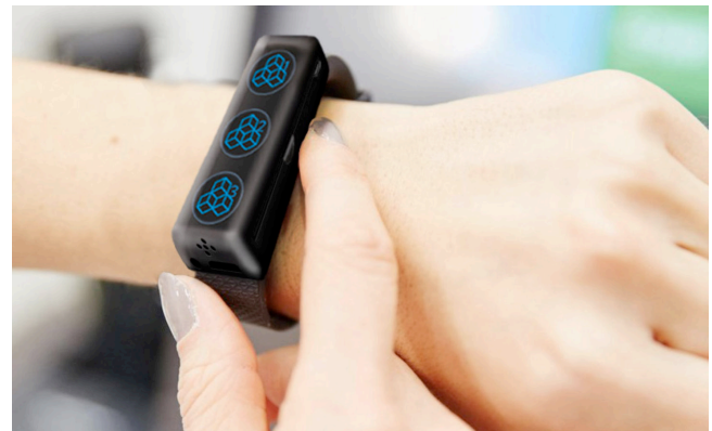
Figure 1. WeaRelaxAble can be controlled from a wrist-worn arm-band. The figure displays a mocked-up rendering of our proposed system. The device is fastened to the arm and can thus capture body data, such as heart rate, skin conductance and heart rate variability. By means of the the blue icon buttons, several feedback modalities can be triggered. Feedback includes vibration at the shoulders, heat at the loins, as well as light and sound. The envisioned device incorporates a roll-up OLED display, which can be expanded from the side.
