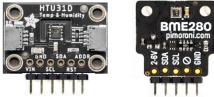
Figure 3.11: HTU31 sensor breakout board by Adafruit and BME280 sensor breakout board by Pimoroni respectively [40, 41].
