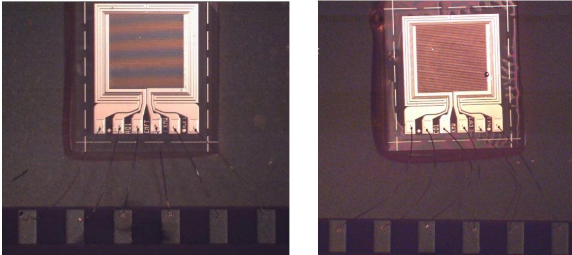
Figure 4.8: Microscopic images of EMFT temperature-humidity sensors A and C after testing for up to 100 hours at 130 °C temperature with 85 % relative humidity inside the HAST chamber.
