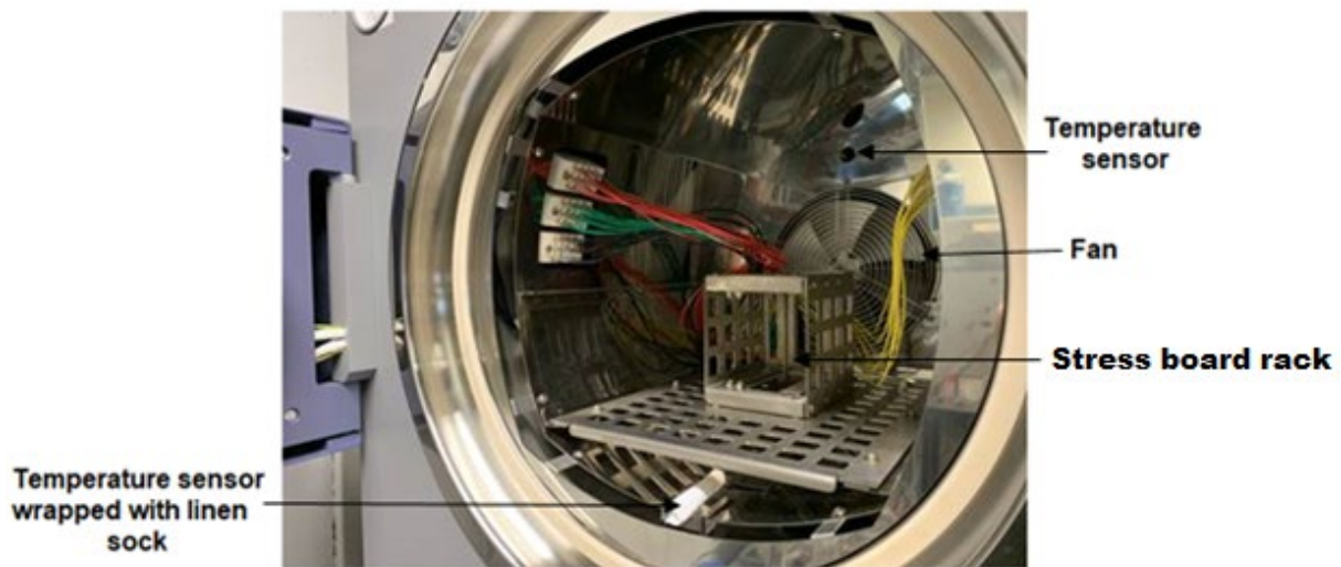
Figure 3.6: Inner view of the chamber of the HAST system EHS-2221MD.
