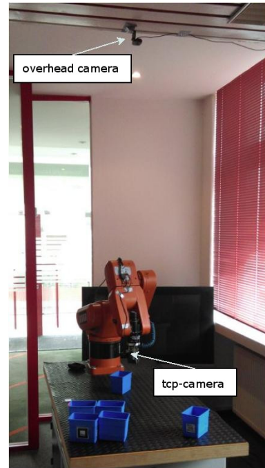
Fig. 1. Construction of the test environment with the robot and the cameras
