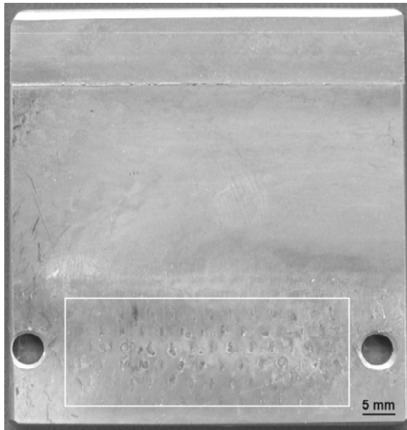
Figure 9: Aluminium die casting plate (white box: position of LTCC/PZT-module)
