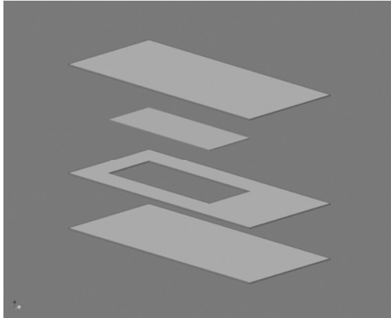
Figure 1: Explosion image of LTCC/PZT-module - without electrical termination; small plate: PZT (schematic)
