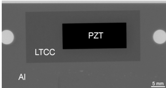
Figure 10: X-ray image of aluminium die casting plate with integrated LTCC/PZT-module
