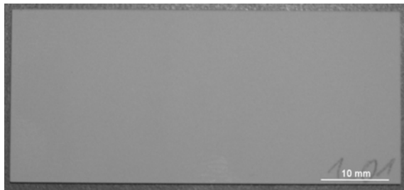
Figure 6: LTCC HL2000 with embedded PZT-plate after sintering
