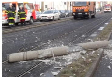
Fig. 1: Broken concrete pole as a result of stress corrosion cracking (source: Main-Post, B. Diem)
