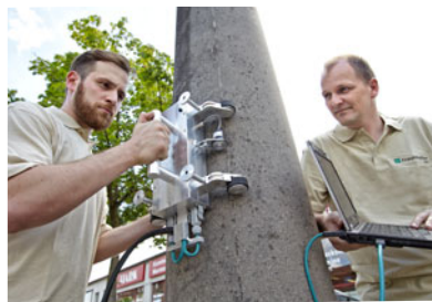
Fig. 5: Mobile inspection system BetoFlux (source Uwe Bellhäuser)
