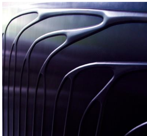
Figure 7: top: extruded absorber with integrated fluid channels [documents from SavoSolar, trade fair "IntersolarSolar2013"], middle: steel absorber [documents from Arcelor Mittal, trade fair "IntersolarSolar2013"], bottom: absorber with bionic design [44]
