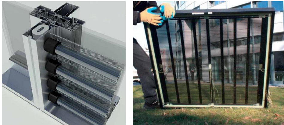
Figure 4: left: vacuum tube collector using a semi-transparent concentrator [14], right: semi-transparent absorber integrated in a glass façade [15]
