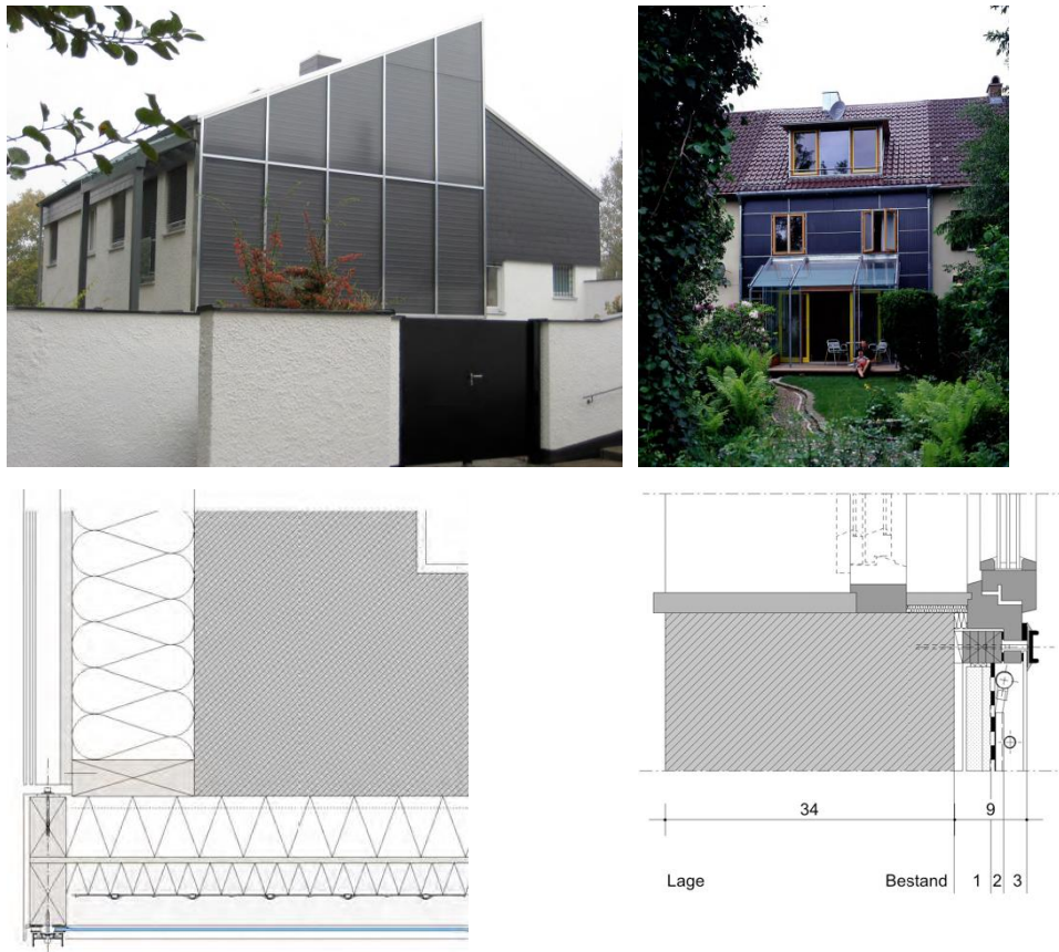
Figure 3: Absorbers integrated in a timber frame construction © Florian Lichtblau, Lichtblau Architekten
