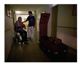
Fig. 6. CASERO having called a care worker after detecting an inhabitant on the corridor during night shift
