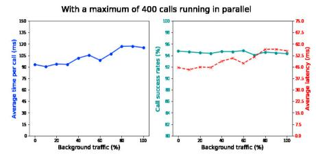
Fig. 4: SIP Call Establishment with a maximum 400 calls in parallel
