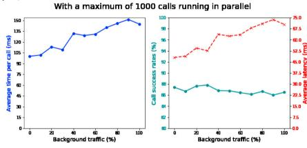
Fig. 6: SIP Call Establishment with a maximum of 1000 calls in parallel
