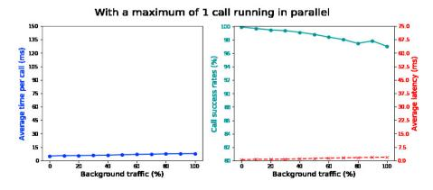
Fig. 3: SIP Call Establishment with maximum 1 call in parallel
