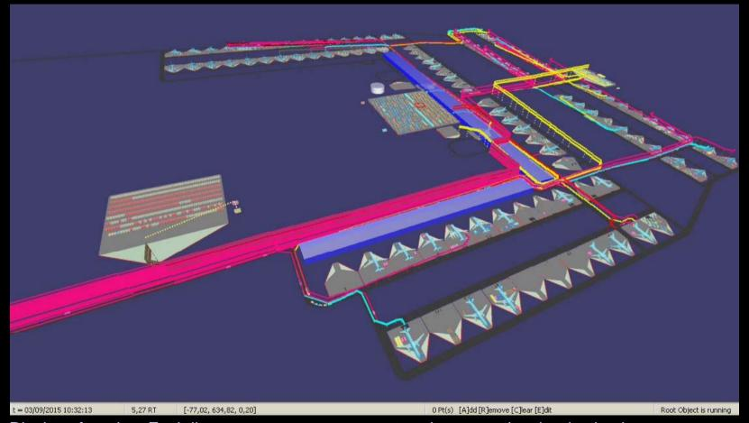
Display of routing: Each line represents one route, stepwise upward to the destination
