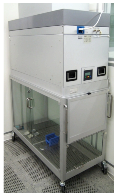
Figure 2. Left: Different flooring material samples for the measurement of the material specific emission rate SER regarding volatile organic compounds VOC according VDI 2083 part 17. Right: Minienvironment with filter-fan-unit, active charcoal VOC filtration and particulate HEPA-filtration, M+W Products GmbH, Stuttgart, Germany.
