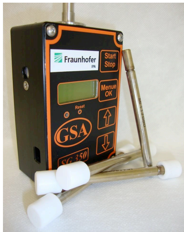
Figure 1. Personal air sampling pump used for sampling of cleanroom air onto Tenax TA sorbent tubes for the determination of the ISO-AMC-Class (VOC) according ISO 14644-8.
