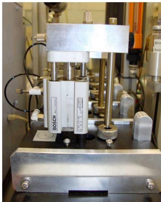
Figure 4. Semi-automated micro-chamber \mu CTE using pneumatic cylinders for the time-controlled insertion and removal of sorbent tubes with appropriate diffusion lock caps from Markes International, Llantrissant, UK.
