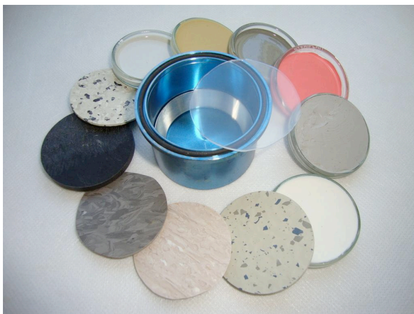
Figure 2. Left: Different flooring material samples for the measurement of the material specific emission rate SER regarding volatile organic compounds VOC according VDI 2083 part 17. Right: Minienvironment with filter-fan-unit, active charcoal VOC filtration and particulate HEPA-filtration, M+W Products GmbH, Stuttgart, Germany.
