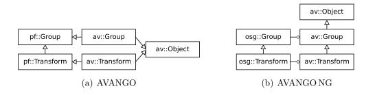
Figure 2: Scene-graph integration in both frameworks
