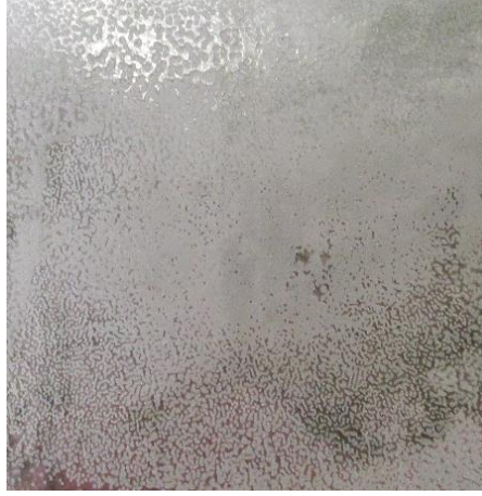
Fig. 3.8 Top plate with glued zirconium dioxide particles ( d_p = 250 \mu\text{m} ).
