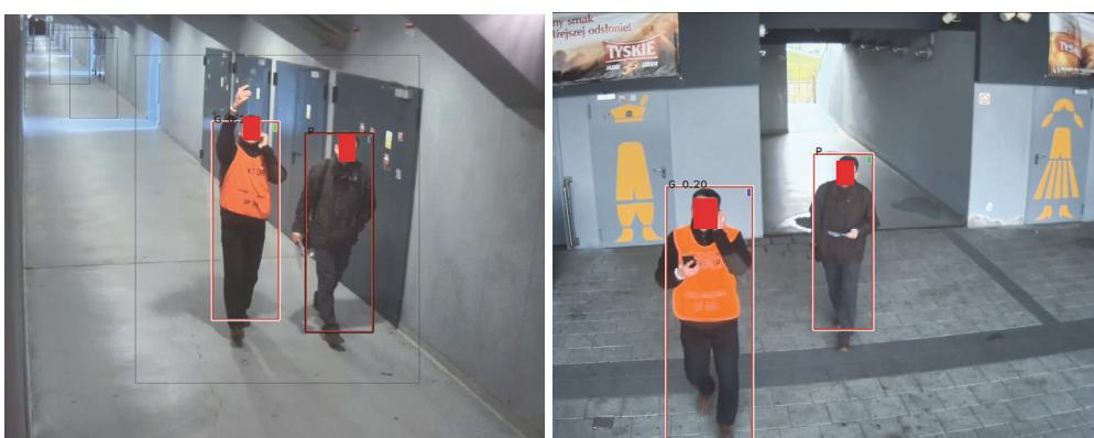
Fig. 3. A security guard and an ordinary person are walking along the hallside inside the soccer stadium. The guard is detected as guard and its position gets logged.
