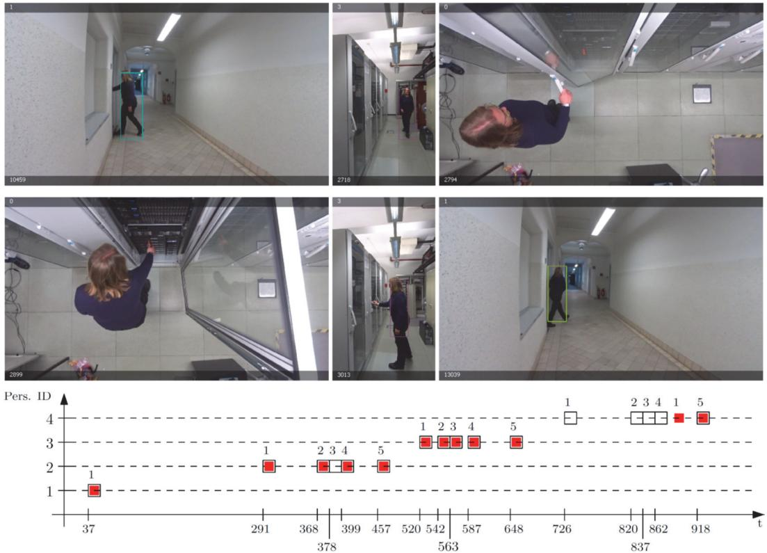
Fig. 2, Qualitative (top) and quantitative (bottom) evaluation in the first scene. The images show the events “enter the server room”, “open server door”, “server manipulation”, “close server door”, and “exit server room”. Unfilled square stands for groundtruth, a filled square represents a detection. From [6].
