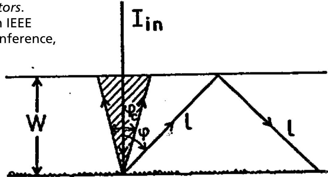
**Fig. 2:** Diffuse back reflector leads to loss cone determined by critical angle for total internal reflection  $\varphi_c$ .
