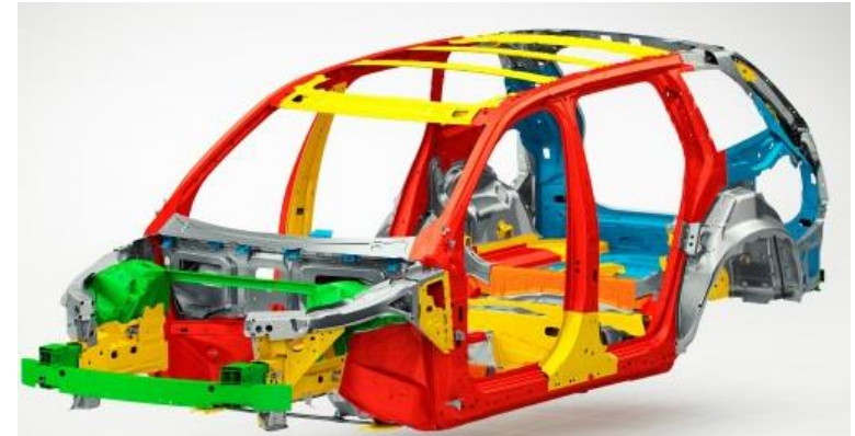
Car body of a Volvo XC 90 (2015) almost 40 % press hardened parts (red), (Source: Volvo)
