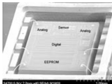
Figure 4: X-ray microphotograph of a bonded pressure sensor
