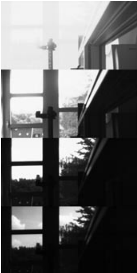
Figure 4: subframes taken with different integration times; total acquisition time: 18 ms
