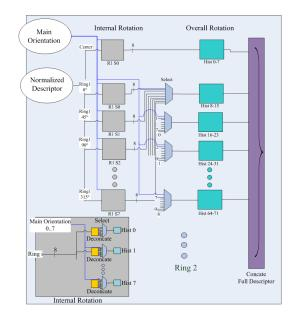
Fig. 6. FPGA Design: Descriptor rotation according to the main orientation. The grey blocks for the internal rotation are detailed in the bottom left corner
