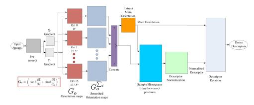
Fig. 5. DAISY Algorithm FPGA Design: Overview
