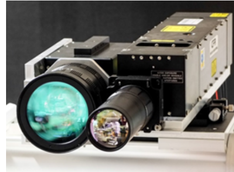
Figure 4. View of the 3D line-detector camera (left) and the laser source (right) equipped with lenses.
