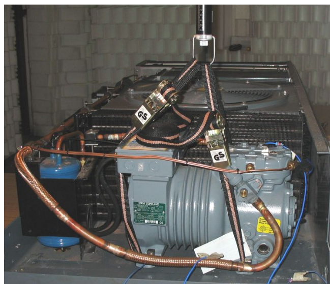
Fig. 3: Compressor suspended from a flexible rope.
