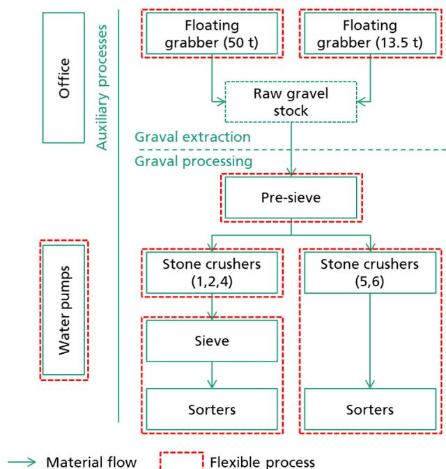
Figure 1 Process diagram of the case study, each node represents a process cluster with electricity demand except for the raw gravel stock which represents only material storage
