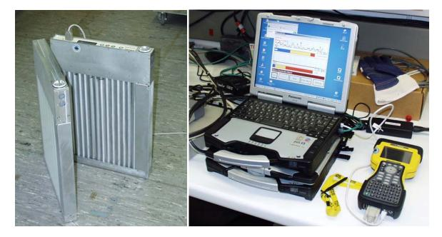
Figure 6: Fission Meter system with detector unit on the left and pocket PC / notebook computer for displaying the measured data on the right.
