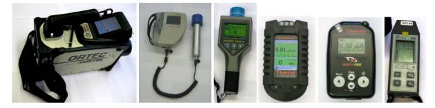
Figure 3: Detectors used for this study, from left to right: Micro Detective [4], InSpector 1000 [5], IdentiFINDER [6], Interceptor [7], RadEye PRD [8], FH40 G-L [9].
