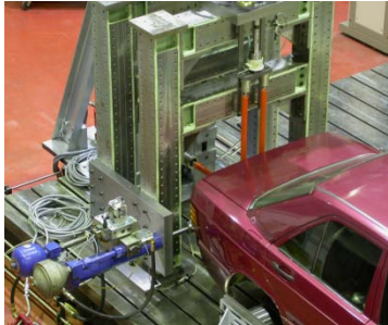
Testing of a trailer coupling device using a multi-axial test rig
