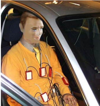
Climate measurement device "DRESSMAN" for the evaluation of thermal comfort. Here inside a vehicle.
