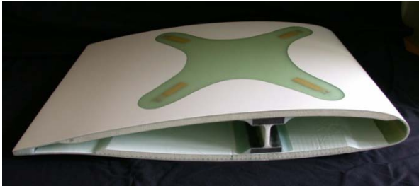
Monitoring system for impact and delamination detection
