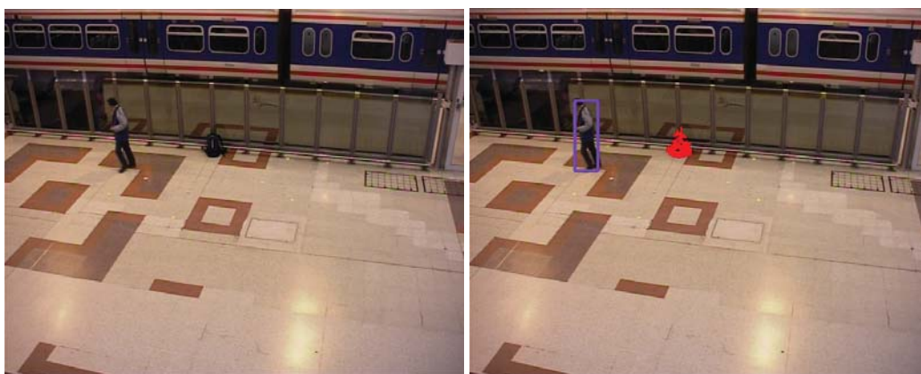
Fig. 4. (Left) Sample input image. (Right) Example of detected abandoned object. (PETS2006 dataset; S1-T1).
