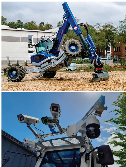
Figure 6: Top: Autonomous walking excavator of DFKI. Bottom: Additional sensors like LiDAR scanner and cameras for various tasks. Photo credit: Felix Bernhard – DFKI Bremen.
