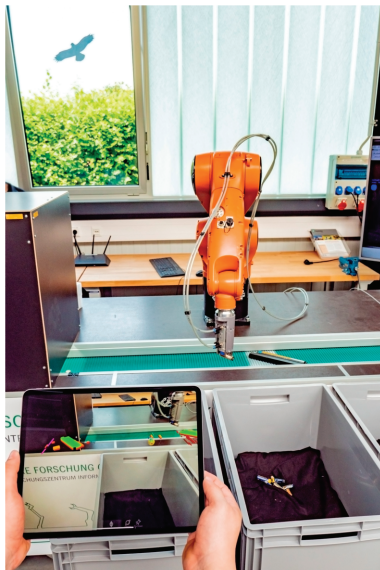
Figure 9: Sorting and classification system by FZI for hazardous waste handling.
