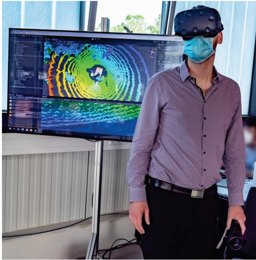
Figure 2: VR telepresence system developed by KIT-ISAS as one example for the ROBDEKON control stations.
