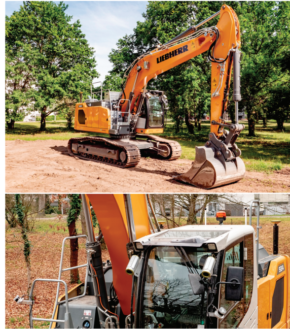
Figure 7: Top: Autonomous crawler excavator of Fraunhofer IOSB. Bottom: Some of the added hardware (GNSS, LiDAR scanners, stereo cameras, WiFi) in greater detail.
