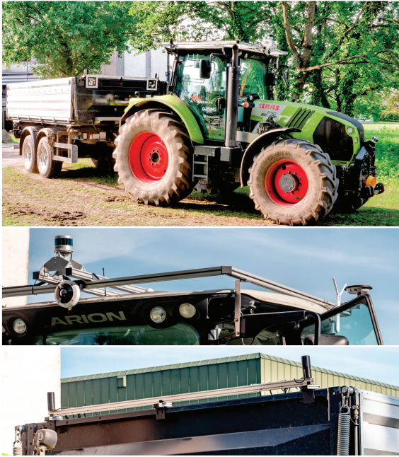
Figure 8: Top: Combination of autonomous tractor and dump trailer of Fraunhofer IOSB. Middle: Additional sensors on the roof: Cameras, LiDAR scanner, GNSS. Bottom: UWB (ultra wide-band) localization system mounted on a frame on the trailer.
