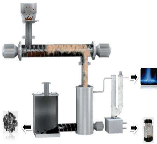
Figure 2: Conceptual drawing of a TCR<sup>®</sup> plant and of the products gas, oil and char
