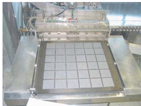
Figure 1: Image of the wafer tray of the industrial PECVD inline system used in this study (Roth&Rau SINA).
