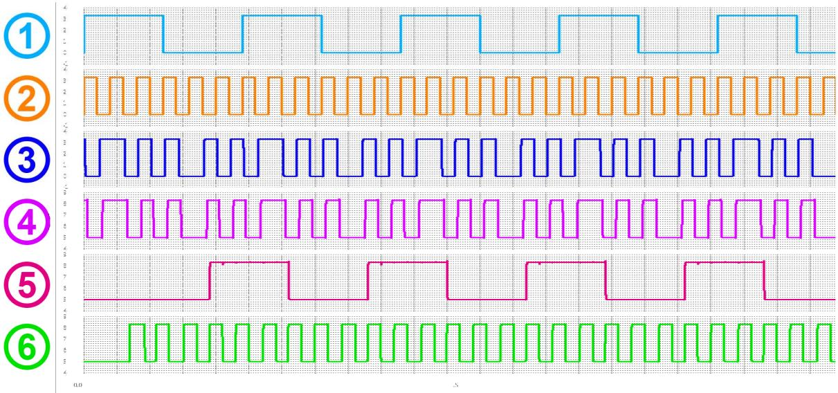
Fig. 9. Simulation of the sequence of encoding, singal conditioning and decoding of the modified Manchester code (1:Data signal 2:Clock, 3:Modified Manchester signal, 4:Modified Manchester Signal after the capacitive coupling element and signal conditioning, 5:decoded data signal, 6:rebuilt clock signal)
