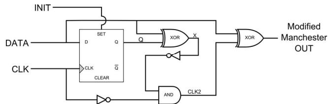
Fig. 4. Modified Manchester encoding circuit
