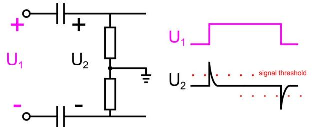
Fig. 2. Capacitively coupled differential signal transmission
