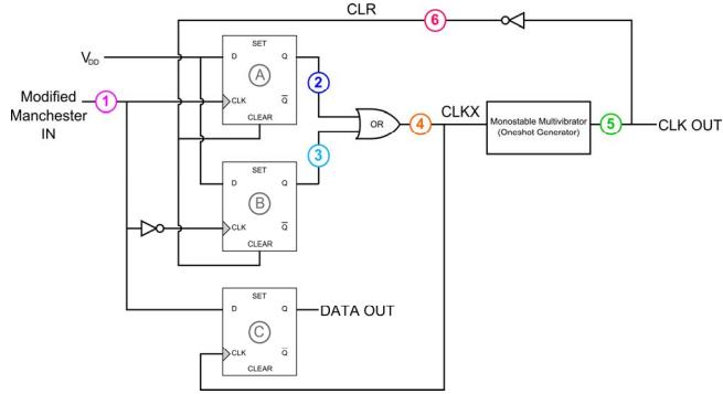
Fig. 6. Modified Manchester decoding circuit
