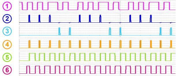
Fig. 7. Simulation of the decoding sequence (1: Modified Manchester Signal, 2:Output Q of flip-flop A, 3:Output Q of flip-flop B, 4: Signal CLK, 5:Signal CLK\_OUT, 6: Signal CLR)
