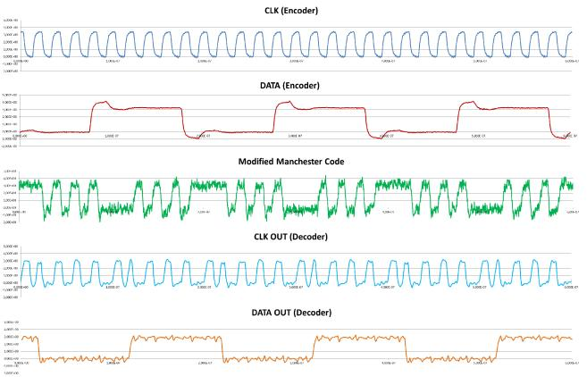
Fig. 8. Measurement of Modified Manchester encoding and decoding
