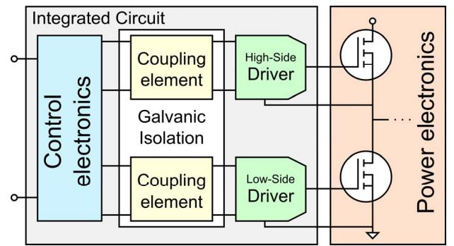
Fig. 1. Smart power converter topology utilizing a galvanic isolation
