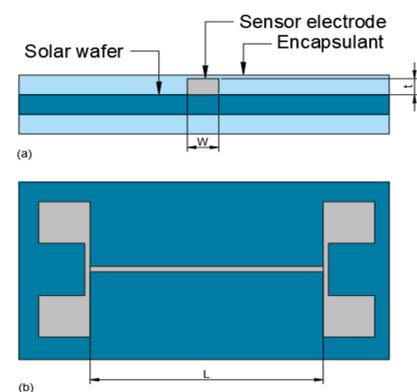
**Figure 2:** Schematic drawing of the temperature sensor with design parameters (a) Cross-sectional view (b) Top view.
