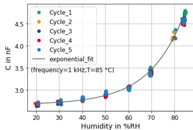
**Figure 5:** Measured capacitance of humidity sensor at 1 kHz with exponential curve fit of the five-cycle test at 85 °C
