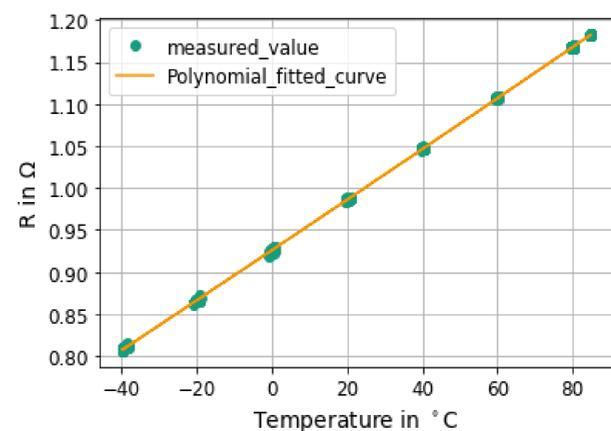
**Figure 6:** Temperature dependent resistance measurement of temperature sensor
