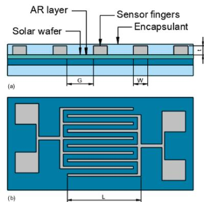
**Figure 1:** Schematic drawing of the moisture sensor with design parameters (a) Cross-sectional view (b) Top view.
