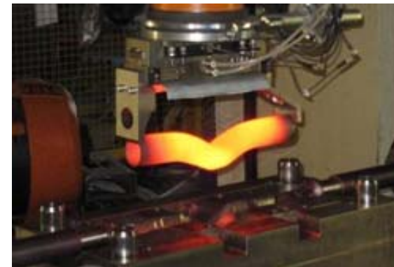
External heated preform
