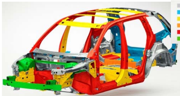
Body in White of new Volvo XC90 app. 40% hot stamping parts (red colored)
