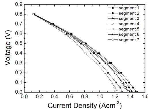
A bistable behavior in the performance of the cell is measured under the steady state condition
