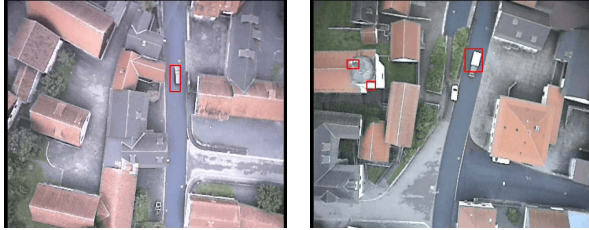
Figure 7 : Detected moving objects are marked with bounding boxes. Due to violation of the 2D-model assumption, the tower of the church was wrongly detected (right).
