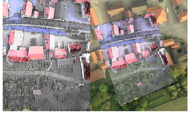
Figure 5 : Registration of a corrupted frame (left) to the orthophoto (right).
