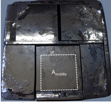
Fig. 1. Photography of one of the investigated blocks. 125x125mm 2 wafers were cut from the lower central brick (“A middle ”) as depicted by the white frame.
