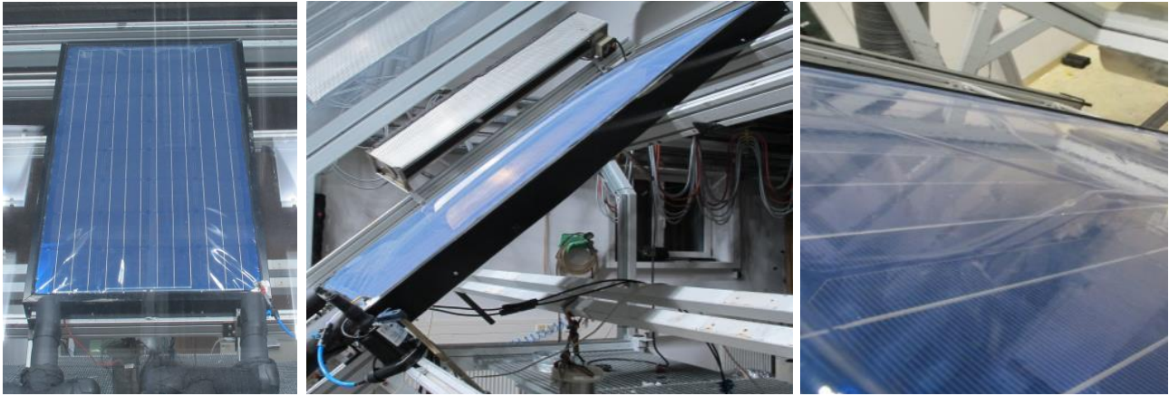
Figure 5.10: Photos of PVT collector with switchable film insulation “PVT04-film” during indoor testing in normal, inflated mode (left and center) and in protected, deflated mode (right).
