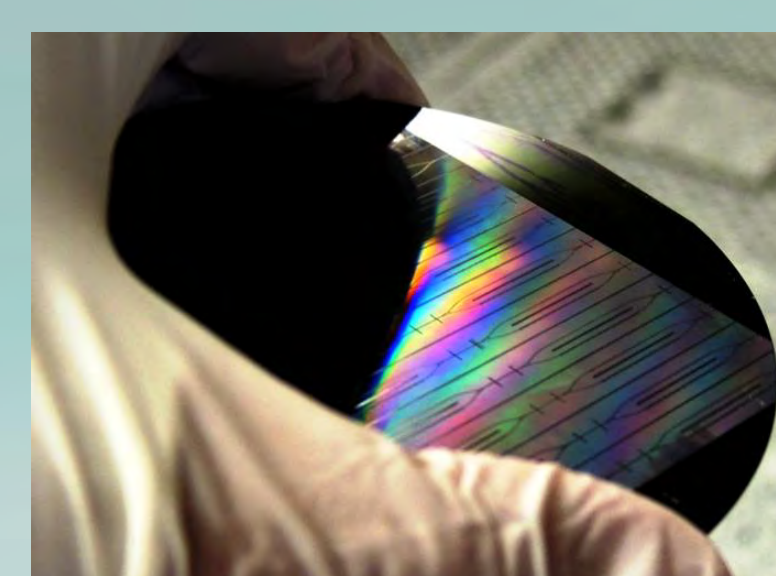
Image of a 100mm silicon wafer containing waveguide structures with surface Bragg gratings imprinted into OrmoComp®.
