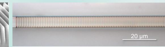
**SEM (left) and optical microscope** (top) image of replicated surface relief grating from pattern type # 3. No defect or structure collapse visible over the whole length.
