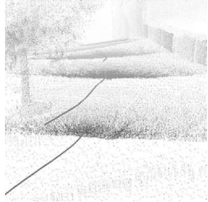
Figure 18: The trajectory after mapping shows gaps, since the robot poses are corrected at 3D scan poses.
