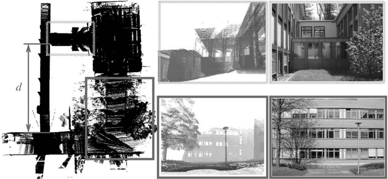
Figure 13: The closed loop with a top viewing position and orthogonal projection. The distance d measured in the point cloud model is 2096 cm, measured by meter rule 2080 cm. The right part demonstrates the change in elevation. Top right: A ramp connecting two buildings is correctly modeled (height difference 1.05 m). The ramp connects the basement of the left building with the right building. Bottom right: Outdoor environment modeling of the downhill part.
