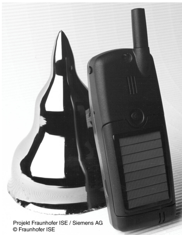
Fig. 4 Cellular phone S25 (Siemens AG) with a photovoltaic module including 8 shingled monocrystalline high-efficiency cells.
