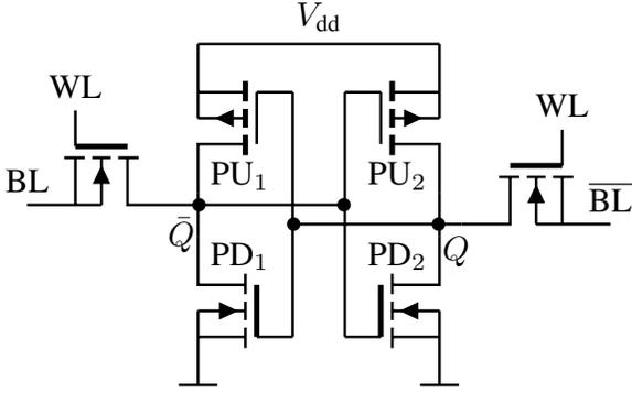
**Fig. 5:** 6T-SRAM schematic. We study the BTI degradation of the four pull-up and pull-down FETs.
