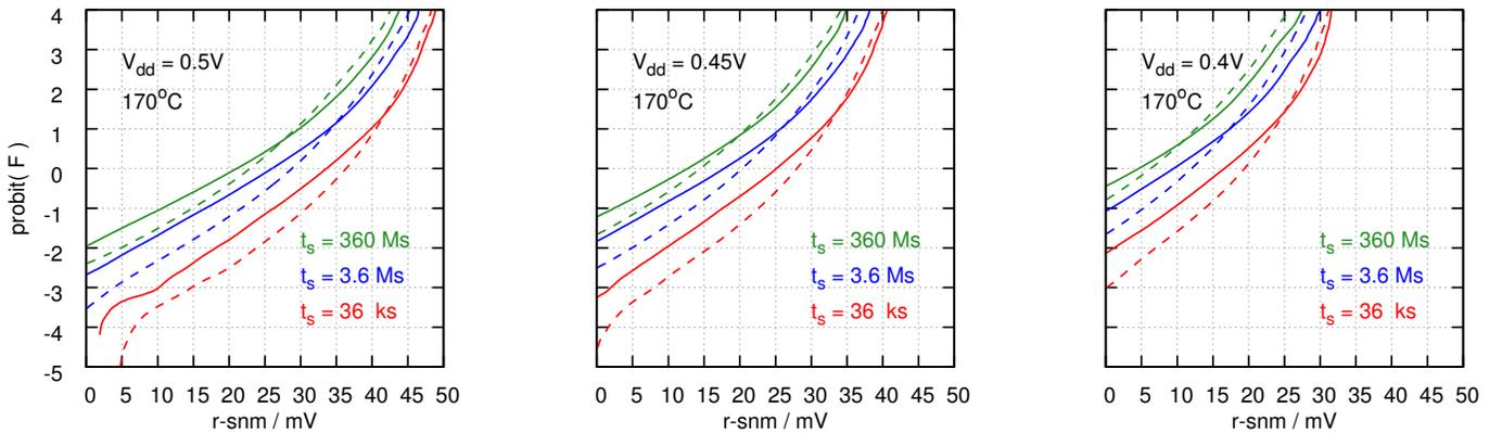
Fig. 9: Read-snm cumulative probability  $F$  for different read- $V_{dd}$  (left to right) and for increasing number of stress periods in the Fig.-3 pattern (bottom-up). Stress patterns with similar effective duty cycle show a different behavior (solid line:  $\lambda_{mic} = 0.99$ ,  $\lambda_{mac} = 0.5$  vs. dashed line:  $\lambda_{mic} = 0.5$ ,  $\lambda_{mac} = 0.99$ ). In particular, there are substantial deviations in the small-snm tail and hence in the cell failures.
