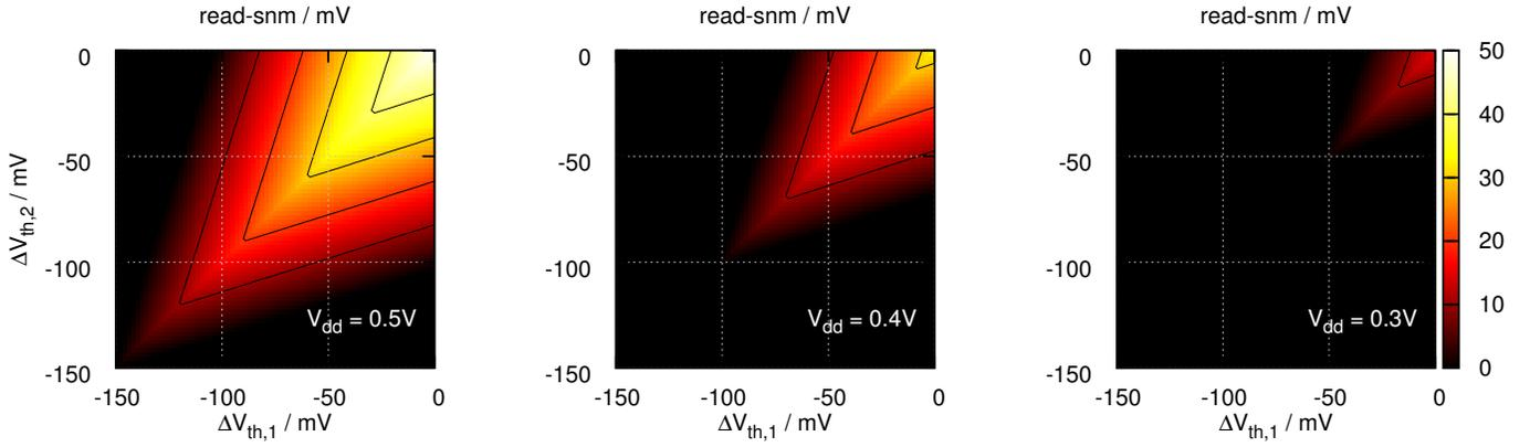
Fig. 7: The SRAM read-snm as a function of the pull-up FETs' shifts  $\Delta V_{th,1}$  and  $\Delta V_{th,2}$ , at decreasing read-phase power supplies  $V_{dd}$  (left to right).
