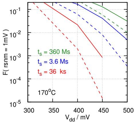
**Fig. 10:** Small-rsnm distribution tail for various  $t_s$  and  $V_{dd}$  (conventions: Fig. 9). The probability  $F(1\text{mV})$  of failing devices at 1mV SRAM noise can differ by a factor of 10...100 between the Fig.-3 scenarios A (solid), B (dashed).
