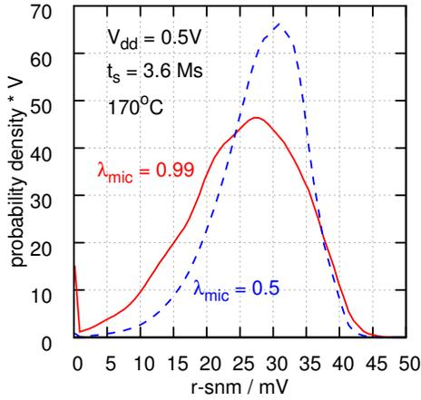
Fig. 8: SRAM read-snm probability distributions after 100  $T_{mac}$  cycles. The Fig.-3 stress scenarios A (solid line) vs. B (dashed line) generate a vastly different SRAM aging, despite coinciding  $\lambda_{eff}$ .
